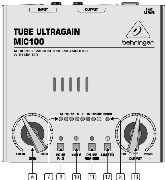
Fig. 2.2: User interface of the MIC100
