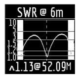
In HAM mode, the SWR icon and the range over which the measurement is carried out are displayed at the top of the screen.
