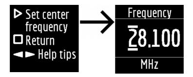
The keys select the cursor position to change units, tens, hundreds, thousands of kilohertz, and the keys change the value. Setting the measurement bandwidth by pressing the keys.
