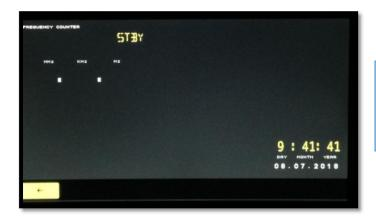
**MENU FREQMTR:** FX773/5 has a digital frequency inside this menu and you can view the operating frequency sampled by the sensor.
