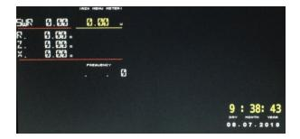
**MENU RZX:** Through this menu it is possible to monitor the paraments R, Z, X, SWR simultaneously.
