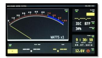
**MENU SMETER:** as a Wattmeter menu but with an analog virtual index. The virtual instrument is autoranging with multiplication factor X. Example if the index indicates 10 and the instrument indicates X100, the measured power is 1000 Watts PeP.
