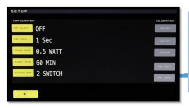
**MENU SETUP:** Through this menu it is possible to set the SWR alarm, time in seconds display PeP power, Trigger watt minimum power for measurements, Sleep Time time for standby, Switch opt number of connected switches. And all the calibrations of frequency, power, swr, on all the operating bands, in more power supply and temperature.
