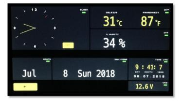
MENU CLOCK: The instrument has a chip dedicated to the system clock and perpetual calendar. It is possible to set the time through the SET submenu. It is also possible to display the temperature and humidity in% of the instrument and the other operating parameters. The sensor is positioned on the back side in correspondence with the ventilation holes.
