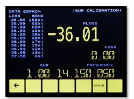
**CALSWR:** through this menu it is possible to recalibrate the SWR part. Connect the radio and set 10W transmit by not connecting any antenna. Caution operation could damage the radio's endings then give a small carrier hit and simultaneously press SAVE button. Repeat this on all 11 bands.
