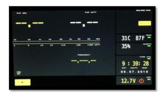
**MENU dBmeter:** here are reported the power measurements in dBm also in graphical format up to 1500 Watts. Possibility to select also CH1 / 2 operating sensor.
