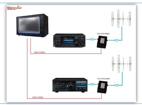
**Connection FX3:** connection scheme to manage HF/50MHz. Through the SMA cables it is possible to interface the Coupler FX3 / 5 and through the EXP bus the two other options can be connected in series.
