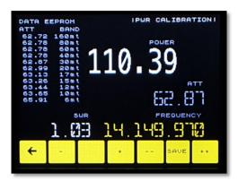
**CALWTT:** through this menu it is possible to recalibrate the AVG power on all 11 bands. The procedure is simple, transmit with 100 Watt on \* dummy load, connect an external precision wattmeter in series to the FX3 / 5 coupler and through the +/- ++ / - keys to match the power read by the FX773/5 Wattmeter with that external reference wattmeter. After saving with SAVE, repeat operation for all 11 bands.
