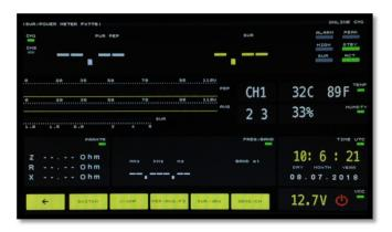
**MENU WATTMETER:** where it is possible to visualize the Power PeP (peak), AVG (average), all paraments SWR, R, Z, X, operating frequency, band, power supply temperature / humidity internal date now select the sensor and antenna switch.
