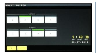
**MENU SWITCH:** through this menu the FX7 antenna switches are managed. If 2 switches are connected, two rows of keys are displayed, one for switch A and the other switch B. If only one FX7 is connected, only one row of keys will be displayed. The green LED indicates the currently selected switch. The settings are stored and retained even after switching off.
