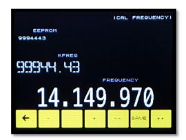
**CALFREQ:** through this menu it is possible to calibrate the internal frequency meter. To transmit with the radio at 10MHz and to set through the keys +/- ++ / - the correct display of the frequency to 10.000.000 MHz to memorize parameter through SAVE key.
