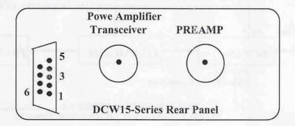
TRX (PA) N(F) - If a Linear Power Amplifier is being used - connect to the Power Amplifier RF Output. If only a transceiver or a transverter is being used, connect to the RF output of the trans ceiver or transverter.
