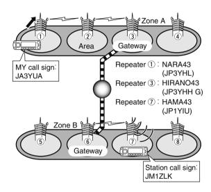
NOTE: If the other station has accessed the repeater at least once, the D-STAR system will connect to the repeater automatically even you don't know where the station is (possible in the same area as you, or in the same zone or a different zone). In this case, you select "GW" as the RPT2 selection. The Auto gateway setting "GW SET" is helpful (p. 136).
