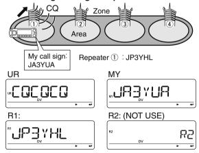
Pushing and holding **[BAND]** for 1 sec. selects the repeater group when in selection mode.
