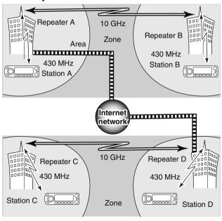
In traditional repeater operation, stations that are communicating must both be in the repeater's operating area. However, D-STAR repeaters can be linked via a 10 GHz backbone, as shown in the illustration at left. Using D-STAR, stations A and B can communicate even though they are in widely separated repeater operating areas.
