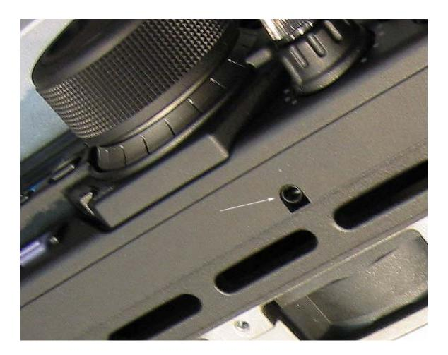
Your FT-Meter requires 12 volts DC at 100 ma to operate the light. Connect a suitable power supply to the  $2.5 \times 5.5 \text{ mm}$  coaxial DC input jack using the provided  $2.5 \times 5.5 \text{ mm}$  jack coaxial power connector (center positive). If you don't want to use the meter light, simply leave the power jack unconnected; the meter itself is a passive device and will work fine without the 12 volt input.
